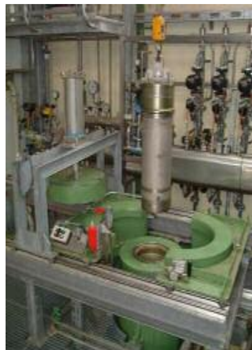
Figure 2: Filling 1000 bar extractor with basket
